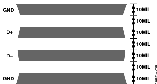
Figure 35. Arrangement of Signal Tracks
